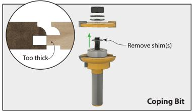
**Solution:** Remove shims from within the tongue space to decrease the thickness of the tongue.
