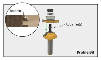
**Solution:** Add shims between the groove cutter and design cutter to increase the height of the design.
