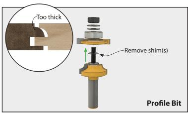
**Solution:** Remove shims between the groove cutter and design cutter to decrease the height of the groove.
